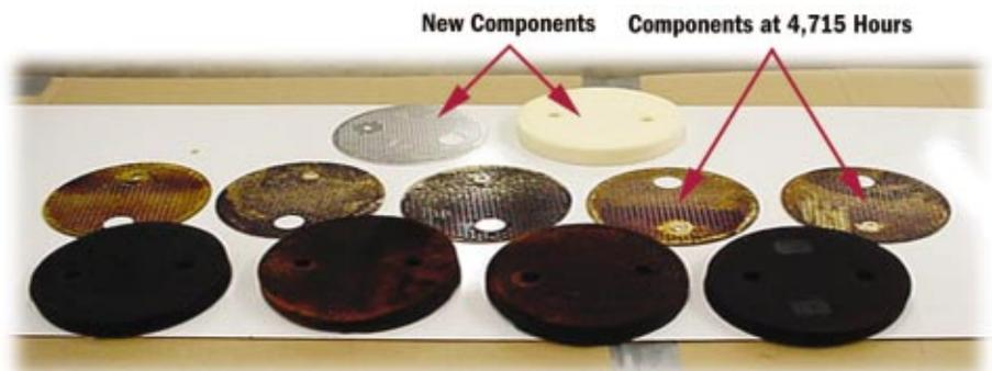
**Figure 1. New and Used Electrostatic Cell Components**
