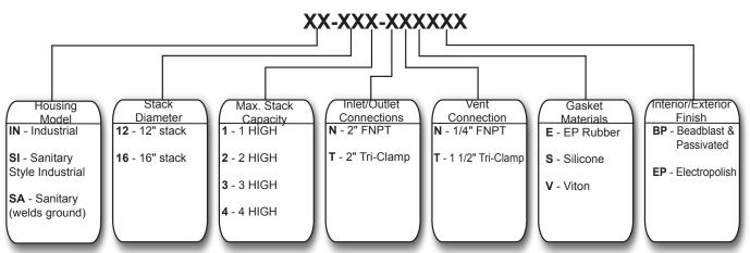
**Example:** To order a standard 12" 1-HIGH Industrial housing with standard connections, gaskets, and surface finish, the order should read as follows: IN-121-NNEBP
