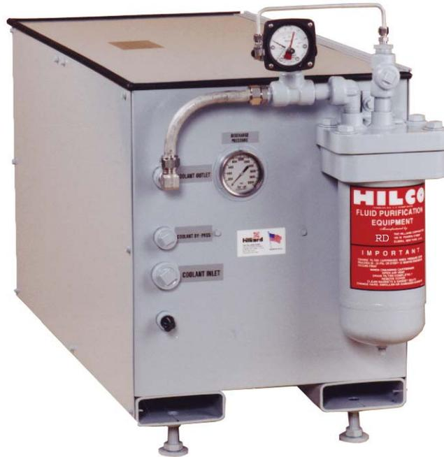
The Hilliard model CA-10-8 "Chips Away" high-pressure coolant delivery system is equipped with a built-in 25-micron absolute high-pressure filter which eliminates any plugging and erosion of the coolant pathways in this critical application. Considering the assembly-line demand of 1000 coil pocket inserts per day and the economic impact of any downtime, this is an extremely important feature.
