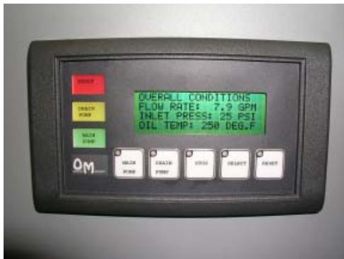
*The local operator interface panel displays the system's operating status at all times.*
