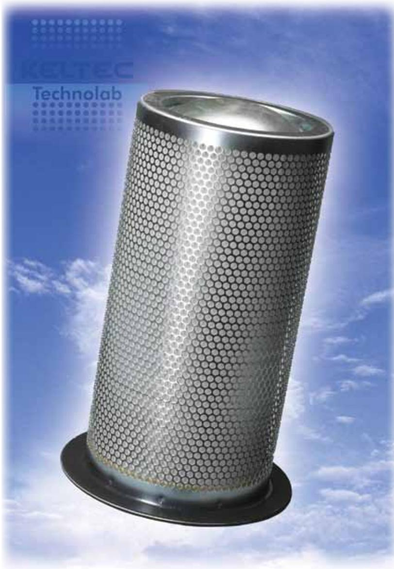
The standard conventional oil separator is the original design for the removal of oil aerosols from the compressed air stream. This element design consists of a specific amount of a uniform grade of borosilicate glass fibers, “wrapped” onto a support tube. When properly sized to the cfm/m<sup>3</sup>/min flowrate and corresponding operating pressure of the machine, this element will provide consistent performance according to the following data:
