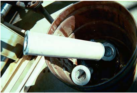
Figure 2. Typical “644” Filters in the waste drum. One new element is seen on top, and a collapsed element is visible at the bottom.
