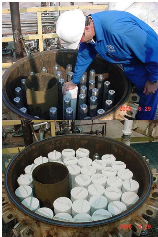
Figure 4. Picture of a typical COMPAX ® Coreless element being installed. The integral handle facilitates the ergonomics of installation.
