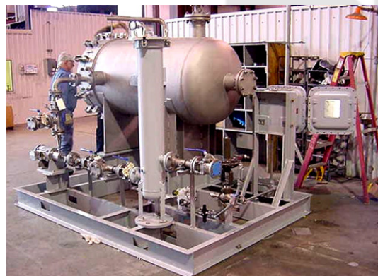
Figure 1: Polarex™ Skid for acid removal from a non-polar fluid
