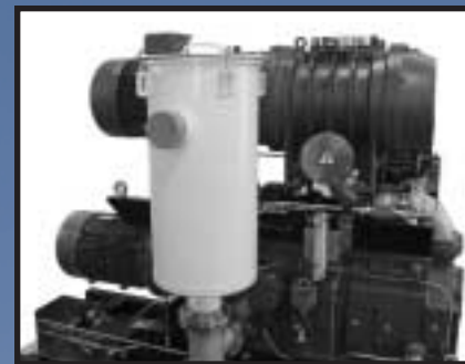
Severe Duty Exhaust Filter on Vacuum Pump
